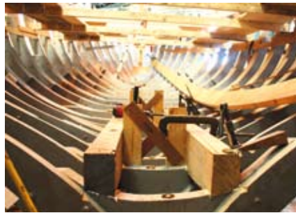
Engine beds and, to right, starboard stringer
