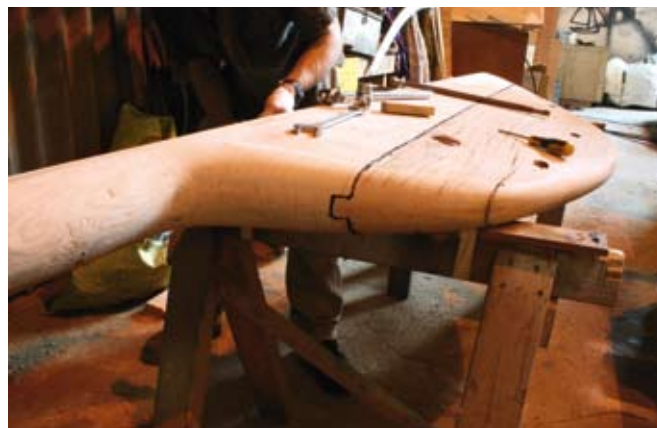
Left: The rudder: two pieces (note the strengthened join) of solid oak
