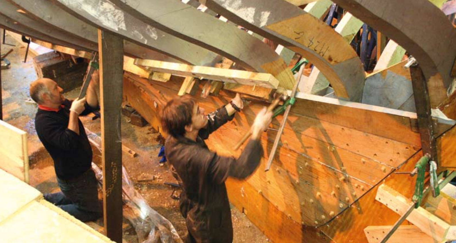
Above: Planking from the bottom up
