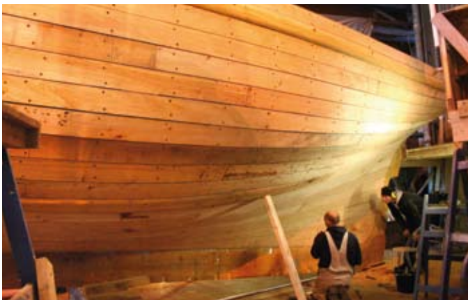
Above: Planking from the bottom up
