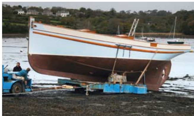
Left: Merlin is positioned at the bottom of the slipway at a low spring tide to await being floated off her cradle by the flood tide
